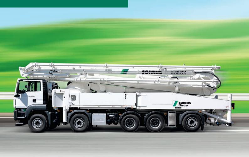
Vertical reach 54.50 m Concrete output max. 162 m³/h Pressure on concrete max. 85 bar
